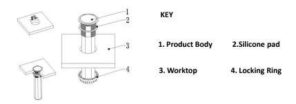
Dimensions: 490mm x 112mm Hole Cut Out Diameter: 95mm Rated Voltage Range: AC95V-250V
